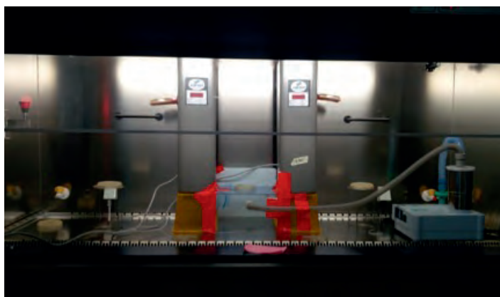
Photo 1: Test set up Air 160, vaporiser and settling plates
